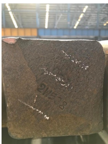
Fig.1. ID is marked by hard stamping on the head cross section surface of the billet
