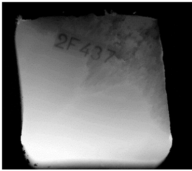
Fig.7. Range map of a billet cross section and demonstrated in grayscale.
